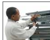
Four 4th-step additions can be stacked on top of the fourth swing-arm then attached securely to the cart frame with buckled straps.
